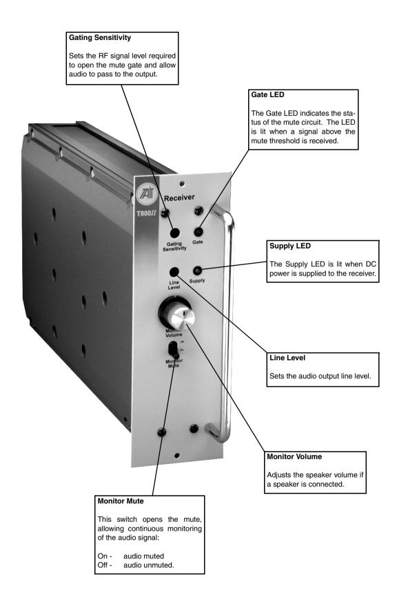
Figure 1.2 T835 Front Panel Controls
