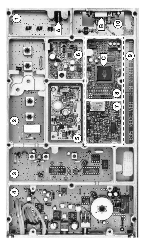
RF input D-range connector ("D-range 1") incl. audio out & DC in (refer to Section 1.2 in Part F) microcontroller microcontroller and CTCSS duct for cabling to extra D-range (if fitted) D-range 8 9 10 A low pass filter receiver front end receiver IF audio processor VCO regulators synthesiser 1284597
